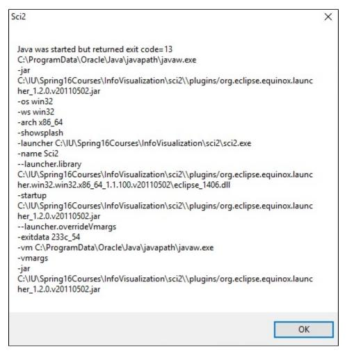
A: The error message that you have received is caused by trying to run Sci2 with the incorrect version of Java required by the tool. For example, if you download the 64-bit version of Sci2, but only have a copy of 32-bit Java installed on your computer, Sci2 will try to run but it will produce this error. To solve this problem, you will need to verify the version of Java installed on your computer.
